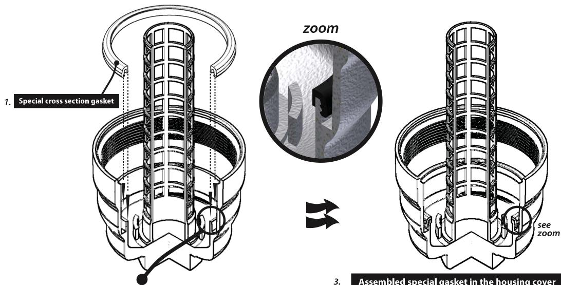
Place for gasket positioning in the housing cover
