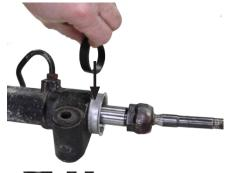
Depending on the model of the steering gear, seals are enclosed.
