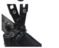
Depending on the type of clamp enclosed, make sure to use the respective appropriate special pliers!
