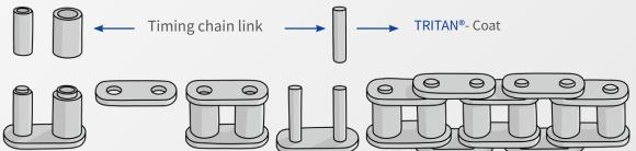
iwis specialists have revolutionised the "TRITAN<sup>®</sup>" PVD (physical vapour deposition) coating technology for timing chain pins and it now withstands these conditions significantly better.
