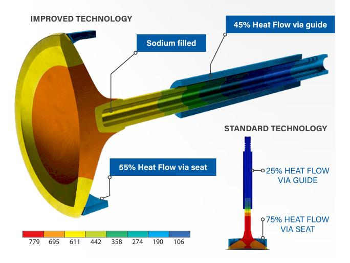
The heat dissipation via the valve guide is improved with sodium-filled valves, which helps to increase durability of the valve. Its hollow structure makes the valve lighter and helps reduce automotive emissions.
