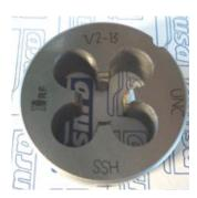
Check the thread type with the metric gauge. Whitworth 1/2-13. Choose the die corresponding with this thread type.
