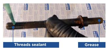
Once these operations have been carried out, **the bolts are ready for their reuse** in the replacement of the cylinder head gasket.
