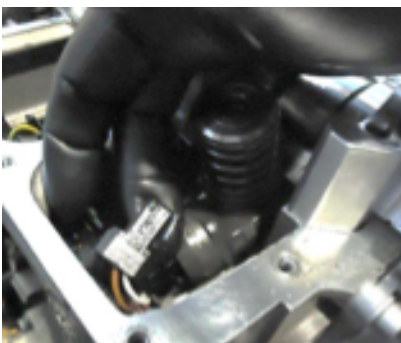
Disconnect electric connector from the injector.
