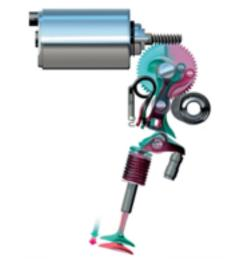
All **intake valves** are linked to an axis actuated by an electric engine electronically controlled, which changes position depending on the engine requirements. Depending on the axis position, **the actuating lever will rest in different positions** on the valve rockers, which will open when the lever receives the camshaft movement at a certain height to allow the mixture.
