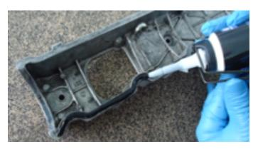
> Place the cover on the cylinder head before the sealant begins to reticulate, this is 10-15 min for AJUSIL. Do not touch any other cord that may damage the cord. The assembly of the valve cover on the cylinder head must be done in one only time.
