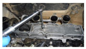
> Tighten the 8 bolts of the cover. Use a torque wrench to apply 0,5 kg. The sequence must begin in the central screw and continue in "X" form outwards.
