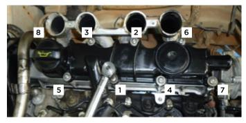
> Assemble the rest of elements removed in the reverse order to disassembly.
