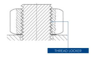
**It protects against vibration**: An internal combustion engine is an important source of vibrations due to explosions are produced inside cylinders. For this reason, the application of Ajulock, with high resistance against vibrations, avoid the loosening (or untightening).
