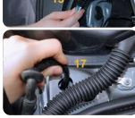
17. Carefully guide cable out of cable routing
