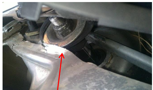
Low quality suspension bearing and insulator assembly
