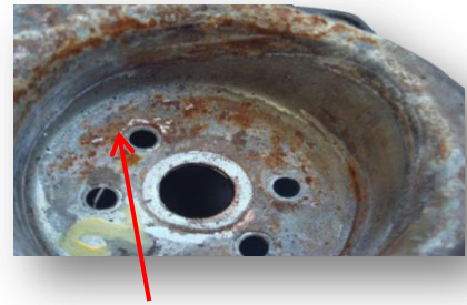
Corrosion caused by movement of the spring
