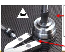
Step 2 : Please respect the recommended clamp tightening procedures according to Ø and/or to the clamp width.
