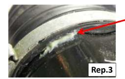
Not enough tightening: Grease leakage
