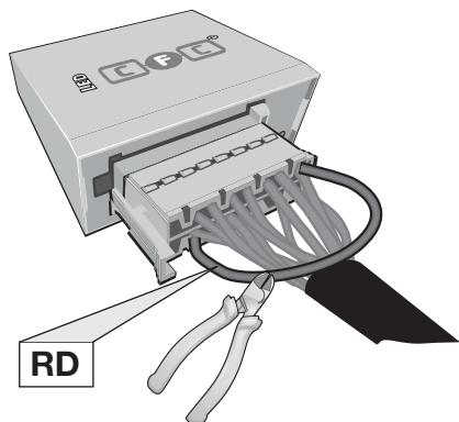
**Pin 11 and Pin 2 disconnected**
