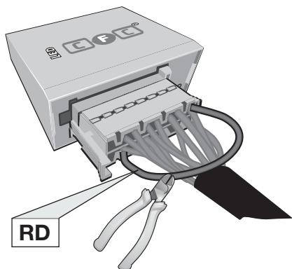
Pin 11 and Pin 2 disconnected
