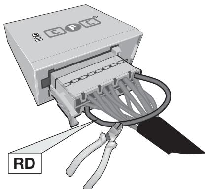
Pin 11 and Pin 2 disconnected
