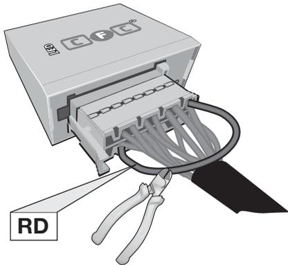
Pin 11 and Pin 2 disconnected
