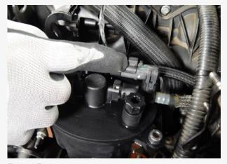
Figure 1 Fuel temperature sensor connector
