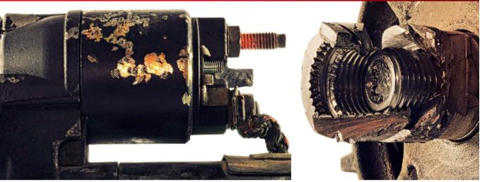
Starter motor damaged by hammer blows Clutch pulley cutted off
