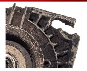
•Broken flange Mounting hole widened and broken
