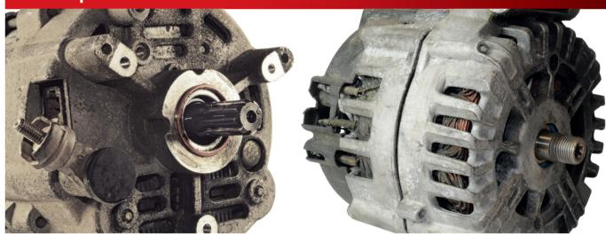
Heavy corrosion on the whole unit
