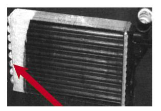
By cars with integrated turbolator heaters the rate of failure by leakage after an exchange increases.
