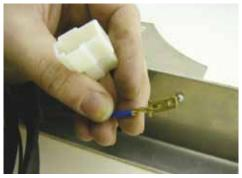
Remove contact plug carefully using a little screwdriver
