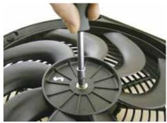
Loosen nut in the middle of the fan Turn fan by 180 °. (Attention: fan
