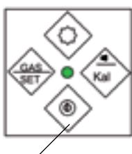
Switching on by pressing this button (only in a gas-free atmosphere). After switching on, the LCD display flashes H2 and HEAt alternately for the duration of the approx. 50 second long heat-up phase. The analogue bar at the lower edge of the display builds up from left to right.
