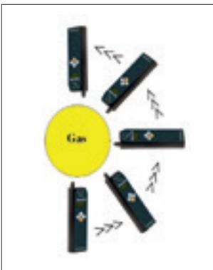
Slow "feeling around" the connection points has proven successful in practice. This is the best way to detect the small bubble of gas escaping.
