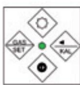
Press and hold the On/Off button for approx. 2 seconds. The device switches on. All the available segments are shown briefly on the display.
