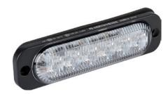
WxHxD: $120 \times 32 \times 14,4 \text{ mm}$ Rated Power:18 WFulfils ECE norm.:R10 + R65Housing Type:Aluminium HousingFitting Position:Left and rightInfo:with sealVoltage:10 to 30 Vwith screws
