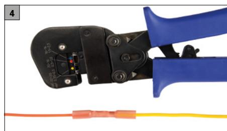
The cables are then crimped with the connector one after the other. In this example with our crimping pliers CrimPro10, alternatively with CrimPro30.
