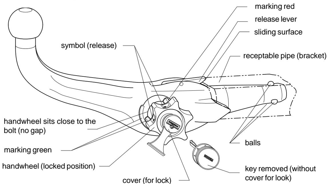
**Unlocked position (coupling hitch unmounted)**
