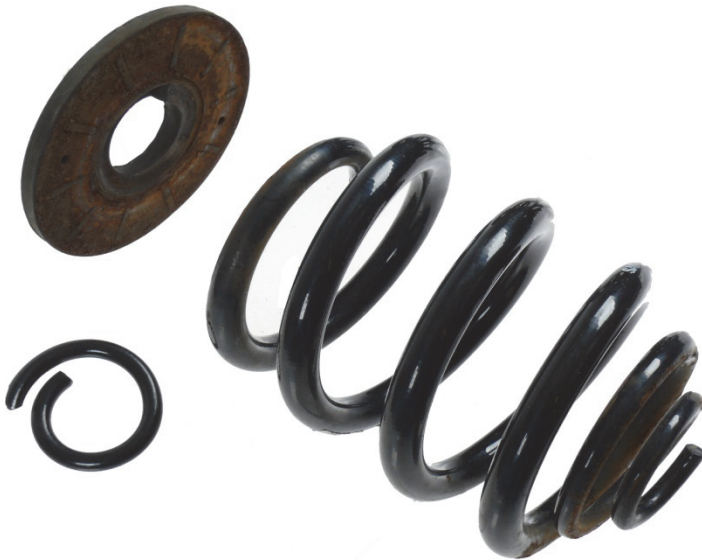
Fig.1: Worn spring seat and broken suspension spring
