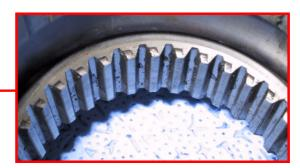
This occurs when the teeth of the drive sleeve do not engage in the hub grooves, but are pushed against the front face of the hub splines. The drive disc is pushed towards the clutch disc in the process.
