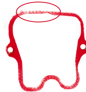
Figure 1 _Compression picture VICTOR REINZ gasket 70-26428-30 (OE 51.03905.0135)
