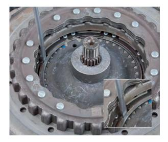
• Remove the retaining ring and clutch disk hub (K1)
