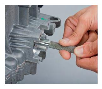
• Coat the lever actuator spindles and the actuator shafts with an extremely thin layer of grease
