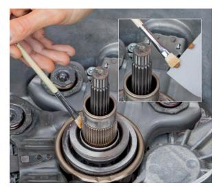
• Moisten the full circumference of the bearing seat of the transmission input shaft with a drop of oil
