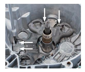
• Remove both lever actuators
