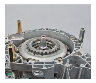
• Fix cross brace (KL-0500-60A) to the threaded bolts using knurled screws (KL-0500-6020A), ensuring that it is not under strain
