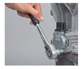
• Remove the servomotors
