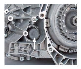
• Mount the transmission on an installation jig or place on a work bench and secure it with the gearbox support (KL-0500-802) so that the transmission is stable and the clutch housing is positioned horizontally
