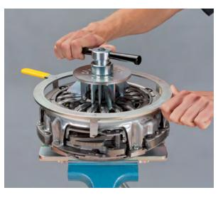
• Remove the clamping nut, locating ring claw fastener and locating ring
