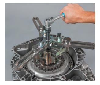
• Remove the clutch assembly with the cross brace
