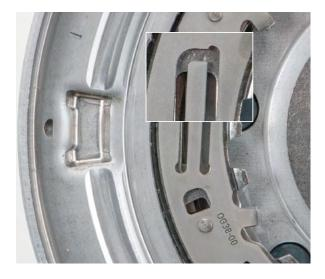
• Position the DMF reset tool KL-0500-8031 at one of the two reset openings on the anti-backlash ring
