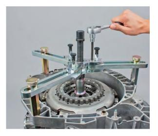
• Press the clutch onto the hollow shaft by turning the spindle above the press-fit sleeve; the press-fitting procedure is complete as soon as the groove for the retaining ring is completely visible through one of the windows in the press-fit sleeve, and the effort required to turn the spindle increases noticeably.
