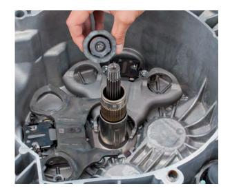
• The middle 4 digits on the return spring and the last 4 digits on the lever actuator must be identical
