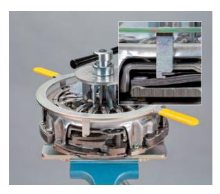
• Rotate the locating ring in an anti-clockwise direction (the direction of the arrow on the ring) as far as it will go and hold
