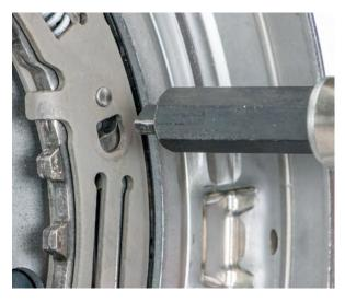
• Turn the reset tool gently in a clockwise direction
