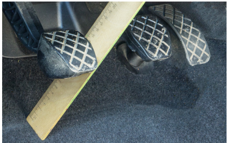
Fig. 1: After the clutch has been replaced, adjust the pedal play.
