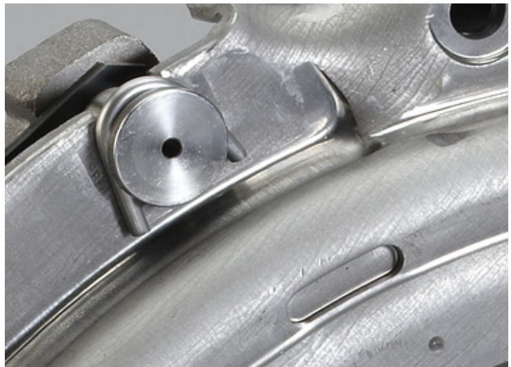
Fig. 2: The wire straps are installed between the stop pins and the clutch housing
