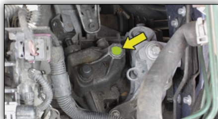
Image 3: Marking on gearbox
