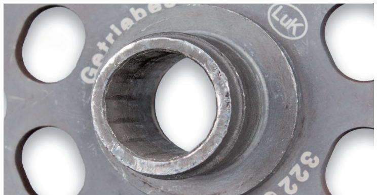
Image 2: Damaged spline profile
