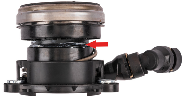
Image 4: CSC damaged by improper installation
