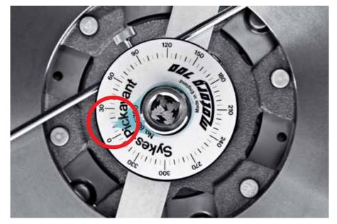
10. Slowly release the slotted arm allowing the arc springs to relax. Read off the degree gauge and compare the measurement against the rated value - see rated value table in Chapter 5.
