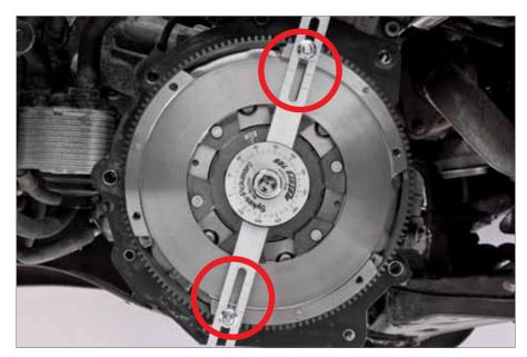
3. Centralise the slotted bar on the adapters by using the graduations and tighten the nuts. The degree gauge must be positioned centrally on the DMF.
