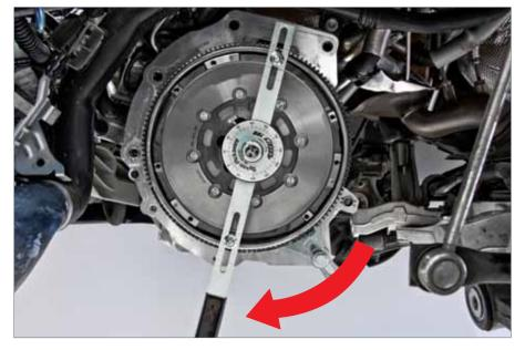
Rotate the secondary flywheel clockwise until the arc spring force can be felt. Slowly release the slotted arm allowing the arc springs to relax.
