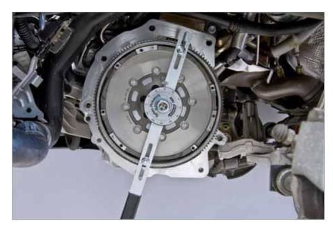
There are a few DMF types with an odd number of mounting threads for the clutch pressure plate making it impossible to mount the slotted bar centrally. In this case, the freeplay angle must be measured by counting the teeth of the starter ring gear – see Chapter 4.3.
