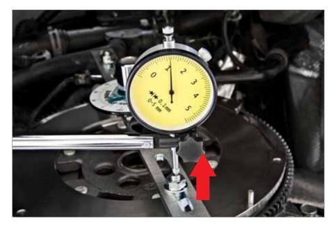
4. Pull the lever gently in the opposite direction (using for example your finger) until res istance can be felt. Read off the dial gauge and compare the measurement against the relevant rated value – see rated value table in Chapter 5.
