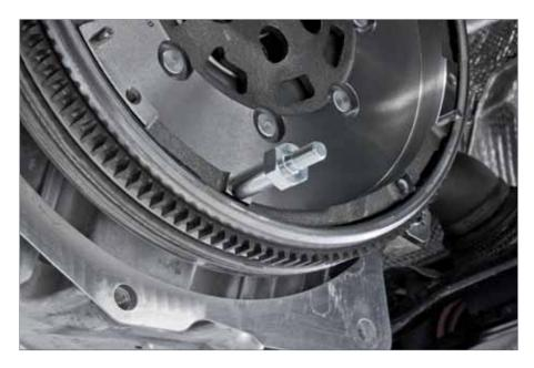
2. Screw the appropriate adapters (M6, M7 or M8) into two approximately vertically opposing clutch bolt holes on the DMF and torque down.
