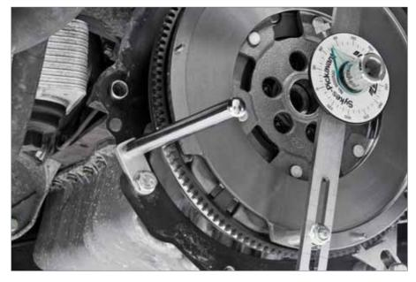
5. Bolt the dial gauge stand to the engine block using a suitable bolt i.e. a gearbox bolt and, if required, the adaptor sleeve can be used similar to the locking tool.
