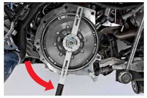
5. Use the slotted arm to rotate the secondary flywheel anticlockwise until the arc spring force can be felt.
