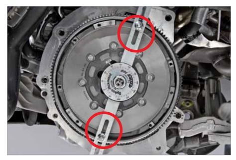
3. Centralise the slotted bar on the adapters by using the graduations and tighten the nuts. As there are an odd number of clutch bolt holes, the slotted arm cannot be fixed centrally on the DMF.
