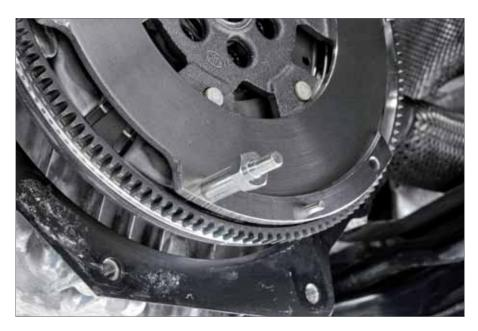
Screw the appropriate adapters (M6, M7 or M8) into two vertically opposing clutch bolt holes on the DMF and torque down.
