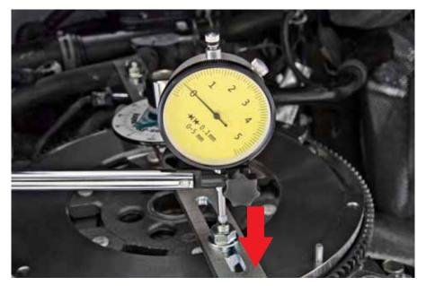
3. Gently push the slotted arm toward the engine (using for example your thumb) until resistance can be felt. Keep the slotted arm in this position while setting the dial gauge to "o".
