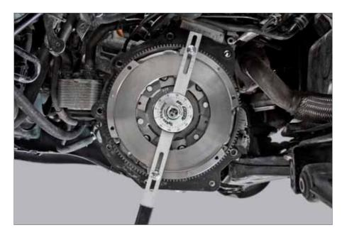
On Dual Mass Flywheels with an even number of threads to secure the clutch pressure plate the slotted bar can be mounted centrally making it possible to determine the freeplay angle using a degree gauge. As this measuring method can be used on almost all DMF types it should be the preferred method – see Chapter 4.2.
