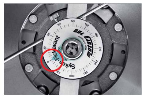
8. Slowly release the slotted arm allowing the arc springs to relax. Set the degree gauge pointer to "o" .
