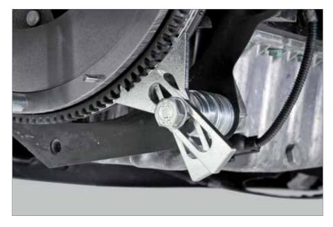
4. Lock the DMF using the locking dogs and, if necessary, appropriate spacers to align the locking tool flush with the starter ring gear.
