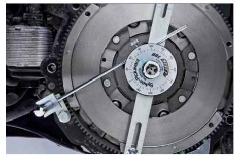
6. Fit the degree gauge locking bar to the degree gauge and the Dial guage stand and tighten the knurled screw.
