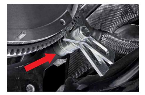
If the locking tool can only be mounted to hole with a dowel fitted, use the adaptor sleeve provided over the dowel
