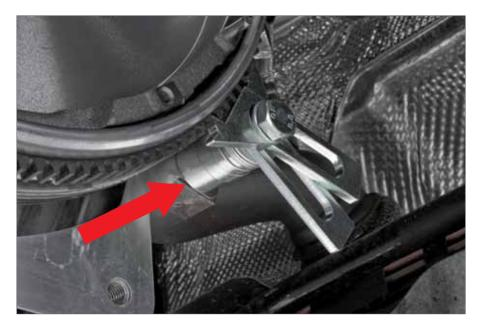
If the distance exceeds the size of the provided spacers, use additional washers. If the locking tool can only be mounted to hole with a dowel fitted, use the adaptor sleeve provided over the dowel.
