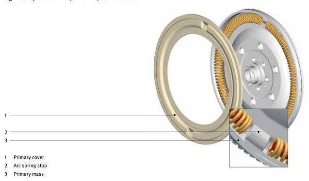
For engine starting, the starter ring gear is positioned on the primary mass. Depending on the type of DMF, it is either welded or shrunk on.
