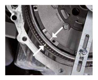
7. Rotate the secondary mass clockwise until the arc spring force can be felt. Slowly release the slotted arm, allowing the arc springs to relax.
