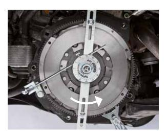
8. Slowly release the slotted arm, allowing the arc springs to relax. Set the degree gauge pointer to "0".
