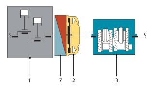
Working principle with a dual mass flywheel
