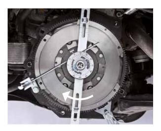
10. Slowly release the slotted arm, allowing the arc springs to relax. Read off the degree gauge and compare the measurement against the rated value – see rated value table in Chapter 8.
