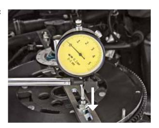
4. Pull the lever gently in the opposite direction (using your finger, for example) until resistance can be felt. Read off the dial gauge and compare the measurement against the relevant rated value – see rated value table in Chapter 8.
