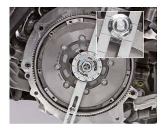
4. Lock the DMF using the locking dogs and, if necessary, appropriate spacers to align the locking tool flush with the starter ring gear.
