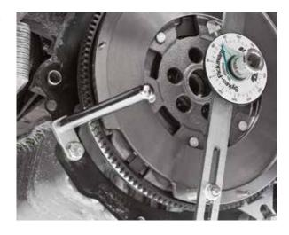
The same bolt can be used to fasten the locking dogs and the dial gauge stand if required.
