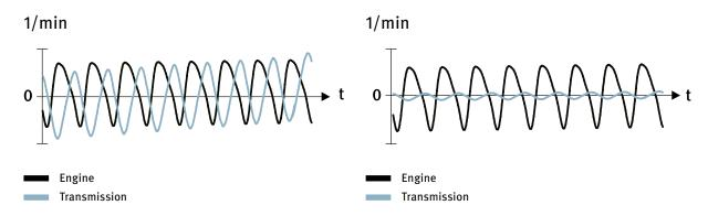
With a conventional flywheel: in the design that was previously common, with a conventional flywheel and torsion-damped clutch disc, the torsional vibrations in the idling range are transferred practically unfiltered to the gearbox and cause the gear teeth edges to knock together (gearbox rattle).
