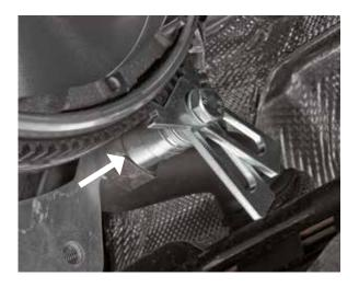
5. Use the slotted arm to rotate the secondary mass anticlockwise until the arc spring force can be felt.
