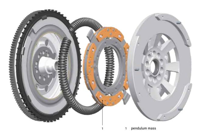
The result is optimum oscillation damping at high torques and low engine speeds. This makes a major contribution to reducing fuel consumption and CO<sup>2</sup> emissions.
