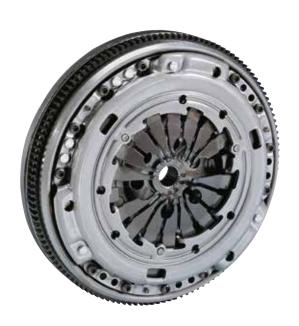
The configuration of the springs in the first-generation DMF was identical to conventional torsion dampers, where the pressure springs are mounted in a radial direction close to the centre and can therefore provide only limited spring capacity. This design was sufficient to isolate vibration in 6-cylinder engines, as these produce low resonance speeds.
