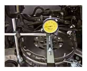
2. Centralise the dial gauge on the adapter and set to the required preload.
