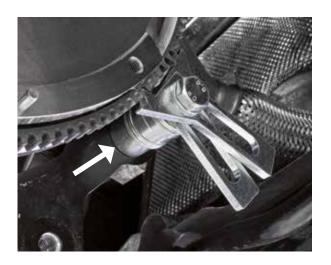
5. Bolt the dial gauge stand to the engine block using a suitable bolt, i.e. a gearbox bolt and, if required, the adaptor sleeve can be used in a similar way to the locking tool.
