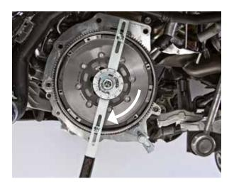
8. Count the number of teeth of the starter ring gear between the original mark and its current position and compare against the rated value – see rated value table in Chapter 8.
