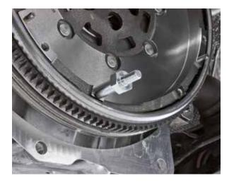
3. Centralise the slotted bar on the adapters by using the graduations and tighten the nuts.
