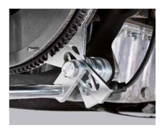
Fit the degree gauge locking bar to the degree gauge and the dial gauge stand and tighten the knurled screw.
