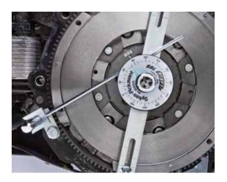
7. Use the slotted arm to rotate the secondary mass anticlockwise until the arc spring force can be felt.
