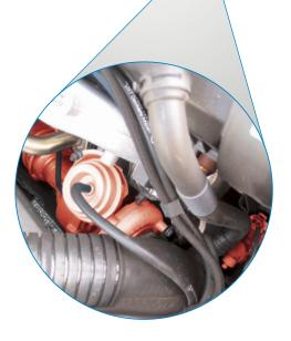
Pressure transducer and VTG charger (highlighted in red) in the Audi A4 TDI
