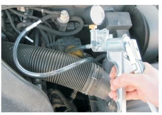
Checking a pressure transducer using a manually operated vacuum pump (VW Golf IV) (Pierburg Art. Nr. 12 00001 11 900)
