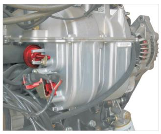
At the controlled intake manifold in the Opel Astra already two switchover valves have been fitted (highlighted in red). One controls through the actuator above it (highlighted in red) the intake manifold throttles; the other switches the secondary air shut-off valve (not shown).
